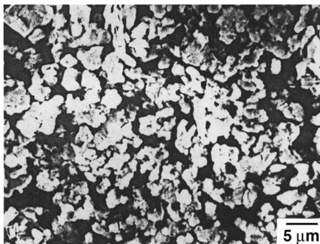
FIGURE 10 The picture of scanning electron microscope of the prepared poly(3-hydroxyaniline).
